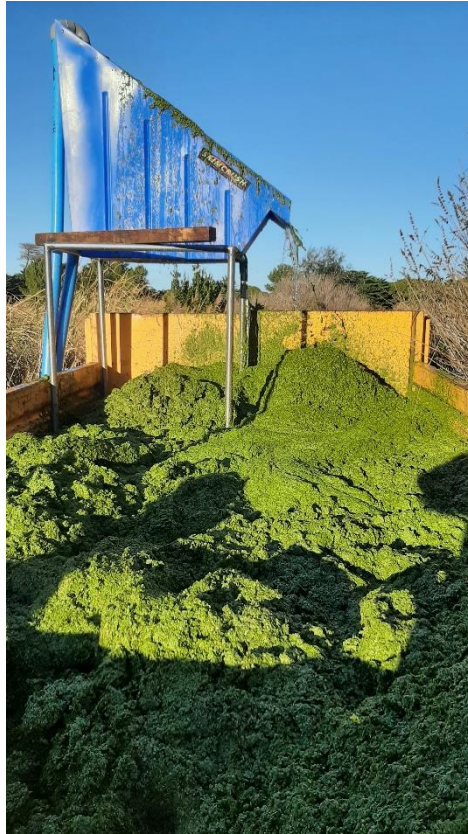
Figure 7. Vacuum device for removal by suction of the duckweed Lemna sp., which is discharged into a container. Photo © Fabienne Tanchaud.
