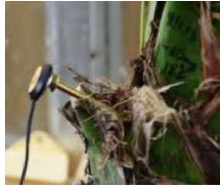
FIGURE 42 : MATERIEL DE DETECTION ACOUSTIQUE EXPERIMENTE A VOLCANI CENTER, ISRAEL
